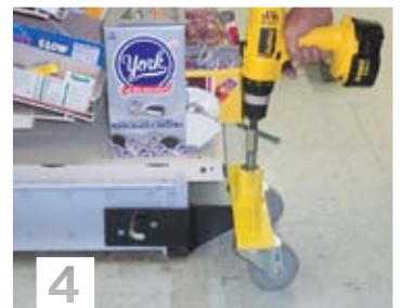
Raise and lower shelving with a cordless drill
